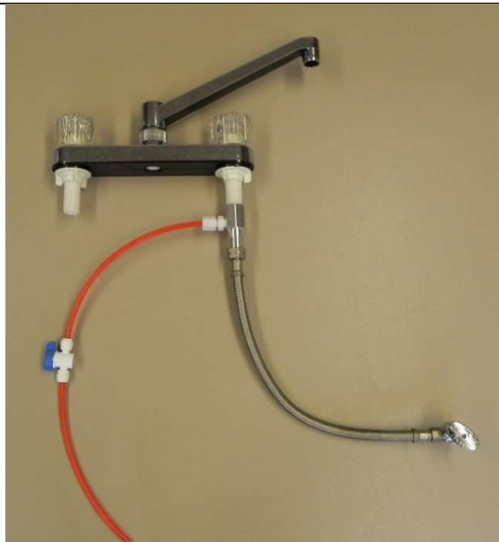
1/2" NPT feed water chrome adapter connect to base of kitchen faucet, with male connector fitting with 1/4" tubing
