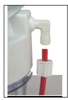
**NOTE:** The system uses compression fitting connections: When connecting tubing to the system, first, you must unscrew the compression nut off the fitting, then pass the tubing through the compression nut about 1", then screw on to the fitting, then use a 5/8" wrench to tighten the nut until the thread is not visible. Don't over-tighten it.
